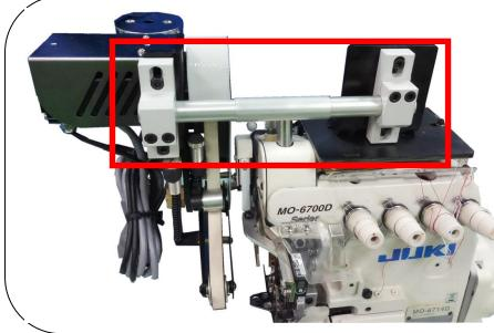
4.裝上支撐架與拖輪 To install the support bracket and puller attachment.
