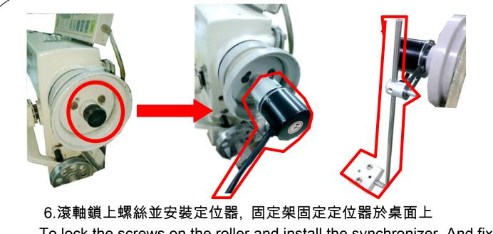
To lock the screws on the roller and install the synchronizer. And fix the synchronizer on the table with the holder.
