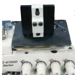
2.放上支撐座並鎖上螺絲 To put the support base and lock the screws.
