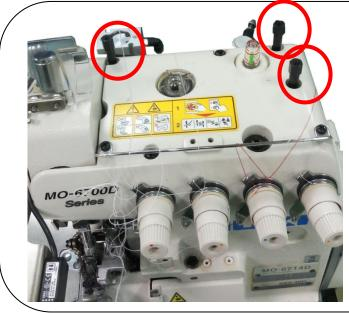
1.更換螺絲並固定 To replace the screws and fixed screws.
