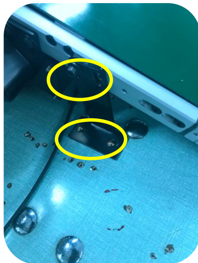
2. 安裝輸送帶 To install the conveyor belts
