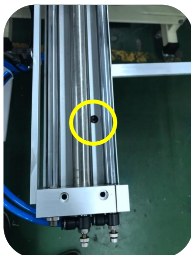
4. 鎖上滑軌支撐架 To lock the fixing frame of rails
