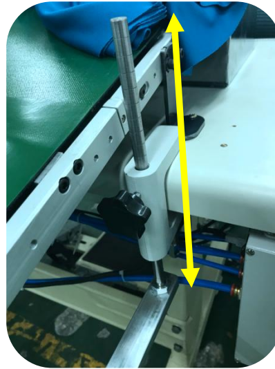
6. 安裝收料區(可調整高度) To install the receiving area (adjustable height)
